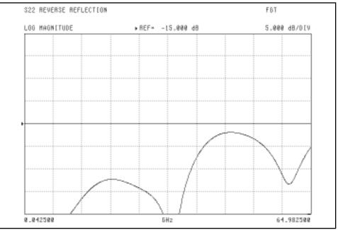
Typical High Frequency Return-Loss measured on VP102F over the range of 40 MHz to 65 GHz.
